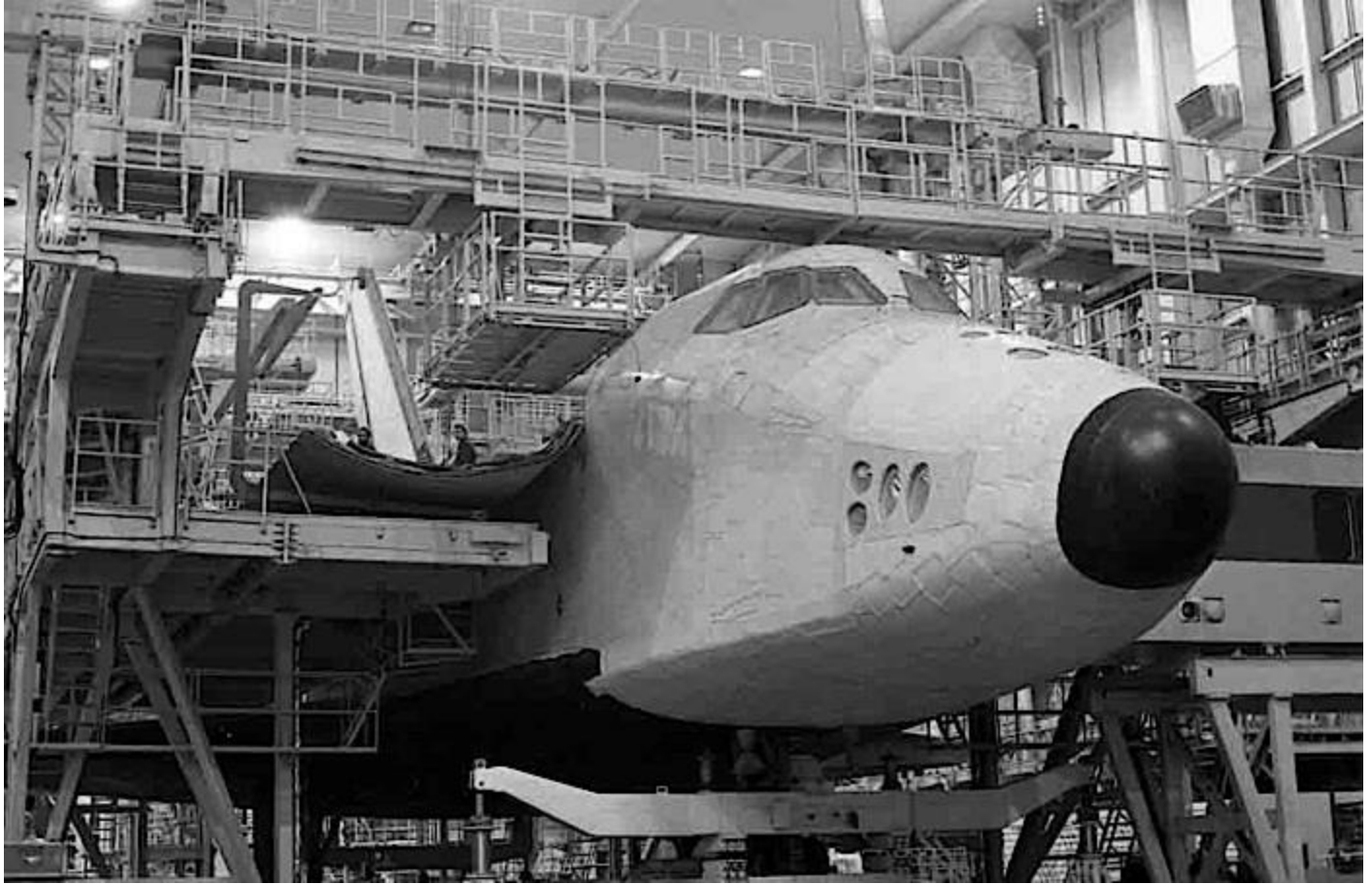
The nose of the fuselage undergoing vibration tests
